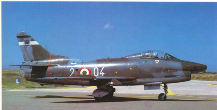
An early Fiat G.91R strike and reconnaissance aircraft wearing the tail badge of the 2nd Stormo from Treviso. The R-model G.91 is powered by a single Rolls-Royce Orpheus engine and armed with four 0.5 inch Colt-Browning machine guns in the nose
