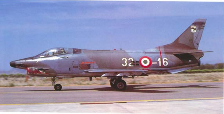
Developed from the G.91R and T-models and built from 1971 to 1976, the more-powerful Fiat G.91Y single-seat light attack aircraft is armed with two 30 mm DEFA 552 cannons in the nose and four underwing pylons for a variety of ordnance. This sharkmouth example from the 32nd Stormo , 13th Gruppo , at Brindisi, is carrying four practice bombs
